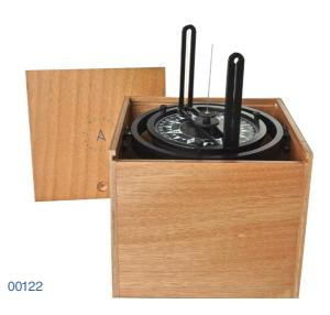
The Boxed Pelorus is stored in its plywood box by resting on two lower gimbals and folding down the aluminium sighting vanes. For operational use, the pelorus is raised to engage two upper gimbals in the box and raising the sighting vanes or installing the sun shadow vane. The plywood box size is 21 x 21 x 18 cm and is finished in natural wood tones.
